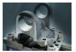
Auxiliary jaws screwed on for optimum machining accessibility and wide clamping ranges.
